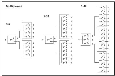
MAXIMUM CONFIGURATION: (8) – Unterminated SPDT relays. (4) – Unterminated multi-pole relays (SP4T, SP6T)
