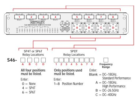
Multipole relay locations A-D: Enter a "4" for an SP4T relay or a "6" for a SP6T relay in the required location. Enter a "0" in unused multi-pole locations. There must be digits in all four positions.
